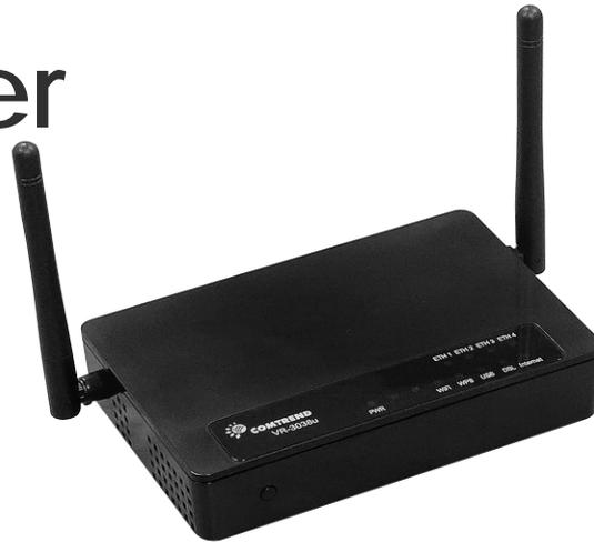
The VR-3038u is an 802.11n compliant Multi-DSL router that supports both ADSL2+ and VDSL2. VDSL2 is a brand new standard and technology perfect for triple play (Video, Voice and Data) applications. The VR-3038u comes with four 10/100 Base-T Ethernet ports, and one USB host, combining wired LAN connectivity and an integrated 802.11n WiFi WLAN Access Point (AP) for wireless connectivity.
