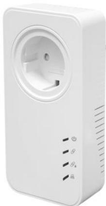
The **PowerGrid 9088**, ITU-T G.hn networking standard compliant ethernet adapter provides the best quality data transmission for the truly high-speed 'connected home' experience. It allows users to extend a local area network via existing power lines, eliminating the need for extra wiring. Installation at home (or in a small office) is quick and easy as the PowerGrid 9088 comes with plug-and-play technology.
