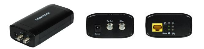
**GCA-6010** is designed as CPE (customer premises equipment) for Ethernet Adapter over coax network home networking, as well as for MDU application over a shared coaxial network. GCA-6010 fully complies with ITU-T G.hn standards for a coaxial interface and supports a 200MHz operating band and built-in diplexer for coexistence of CATV/UHF/VHF services.
