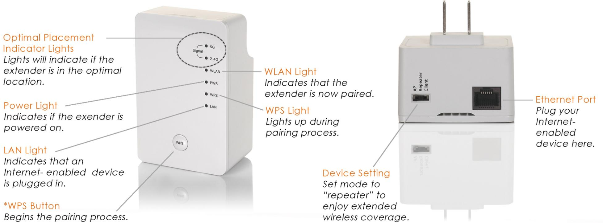
\* If you wish to reset the extender to factory default settings (clear all settings), press and hold the “WPS” button for 10 seconds.
