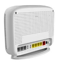
Comtrend's VI-3205u is a Multi-DSL wireless IAD using the updated silicon platform that not only provides both ADSL and VDSL but also supports 5 Giga Ethernet ports. It supports WLAN 802.11n 2.4GHz frequency band and 802.11ac 5GHz Frequency band. Therefore, VI-3205u is designed for high speed applications and is suitable for triple play services.
