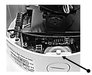
7. Make sure to keep the network camera cover closed and the network cable output is at its correct location.
