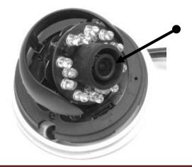
4. Connect this network camera to a \*PoE switch, PoE injector, or DC 5V adapter. Make sure all connection is stable.
