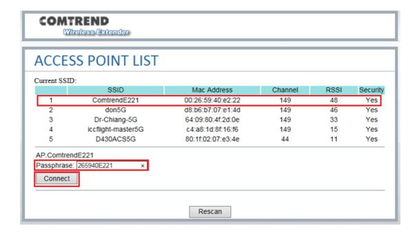
5. To confirm that the connection is sucessful, check that the current SSID is the same as the one that you tried to connect to in the previous step.
