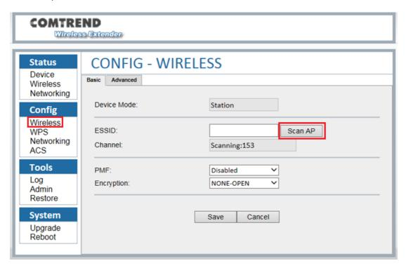
Select an SSID (AP unit) and input the passphrase. The SSID and passphrase (WiFi Key) can be found a label on the bottom on the Wireless Video Bridge. Next, click "connect."
