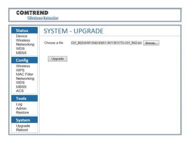
When the firmware has been upgraded successfully, you will be automatically directed to the reboot page.
