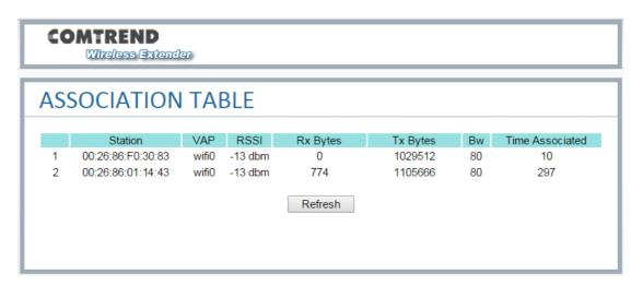
In above example, STA with MAC address 00:26:86:F0:30:83 and 00:26:86:01:14:43 are currently associated to the primary interface (wifi0), If more MACs are listed, more STA are connected with the wifi0.
