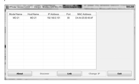
2. If you need to change the camera's IP address, click 'Change IP' button on your selected camera to change the camera's IP address.
