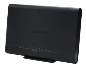
WR-2406u is a FTTH router which provides one RJ-45 for 2.5Giga Ethernet WAN access, one 2.5Giga Ethernet port for LAN access and three Giga Ethernet ports for LAN access. The Wi-Fi 6 device exhibits the best end-user experience with the fastest Wi-Fi speeds, up to 4-times greater network capacity than Wi-Fi 5. The two wireless bands (2.4GHz & 5GHz) are separated in two dedicated Wi-Fi networks, supporting more end-user devices while reducing signal interference.
