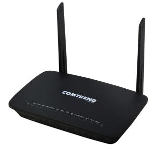
VR-3061u is a Multi-DSL router using the BCM 63136. It not only provides both ADSL and VDSL but also integrated 5 Giga Ethernet ports and WLAN 802.11n 2.4GHz frequency band and 802.11ac 5GHz Frequency band. Therefore, VR-3061u is designed for high speed applications and is suitable for triple play services.
