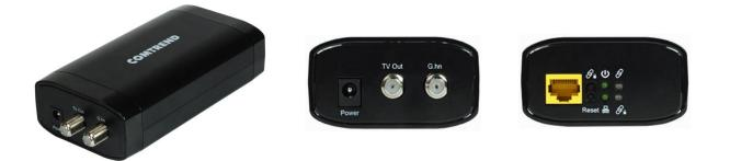
**GCA-6010** is designed as CPE (customer premises equipment) for Ethernet Adapter over coax network home networking, as well as for MDU application over a shared coaxial network. GCA-6010 fully complies with ITU-T G.hn standards for a coaxial interface and supports a 200MHz operating band and built-in diplexer for coexistence with CATV/UHF/VHF services.
