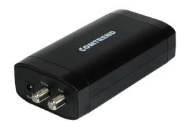
GCA-6010 is designed for the CPE (customer premise equipments) for Ethernet Adapter over coax network for home networking, as well as for MDU application over a shared coaxial network. GCA-6010 is fully complies with ITU-T G.hn standards for a coaxial interface and supports a 200MHz operating band and built-in diplexer for coexistence of CATV/UHF/VHF services.
