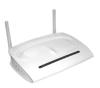
AR-5315u is an 802.11n (300Mbps) Wireless ADSL2+ router comprising four 10/100 Base-T Ethernet ports, a Wi-Fi Protected Setup (WPS) button, a USB Host, and is backward compatible with existing 802.11b (11Mbps) and 11g (54bps) equipment.
