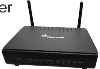
The VR-3033u is an 802.11n compliant Multi-DSL router that supports both ADSL2+ and VDSL2. VDSL2 is a brand new standard and technology perfect for triple play (Video, Voice and Data) applications. The VR-3038u comes with four 10/100 Base-T Ethernet ports, one USB host, combining wired LAN connectivity and an integrated high power 802.11n WiFi WLAN Access Point (AP) for wireless connectivity.
